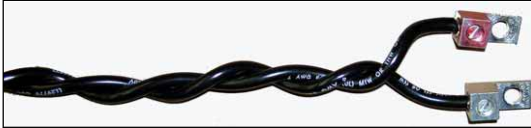
Figure 6 – One end of a #6 twisted pair with a twist of 2.5”
