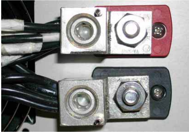
Figure 3 – Typical high-current electronic load cable connections
